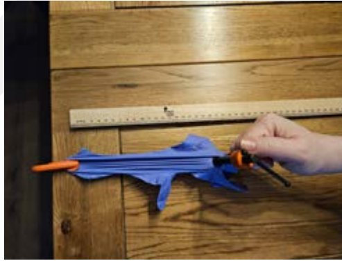
4. Measuring stretched material with ruler
