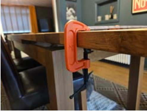
G-clamp attached to table
